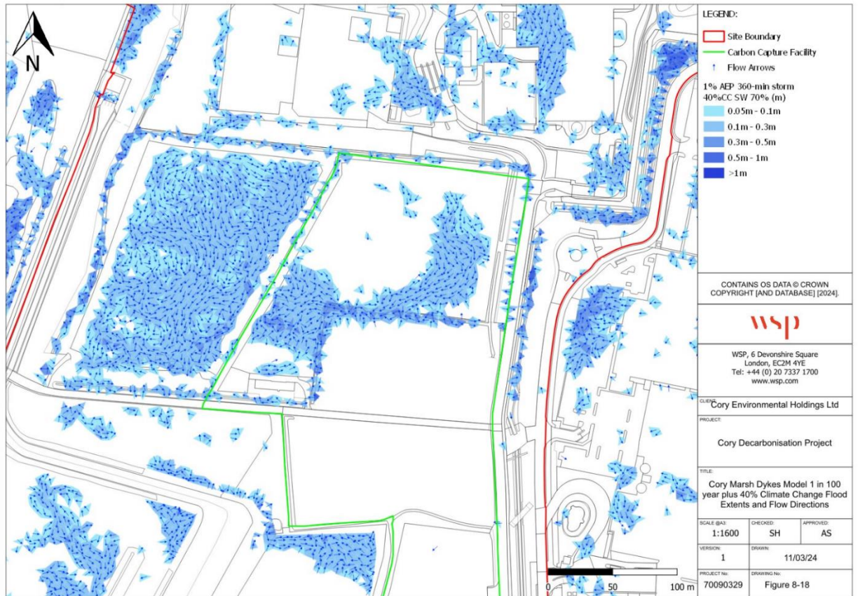
Figure 8-18: Cory Marsh Dykes Model 1 in 100 Year Plus 40% Climate Change Flood Extents and Flow Directions
